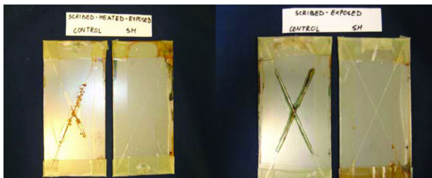
Figure 13. Corrosion test panels: Control and SH- (a) scribed/heated/exposed; (b) scribed/exposed.
